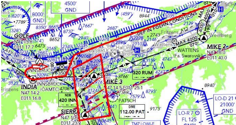
Föhn arrival (red line) along the Nordkette (Seegrube) and avoiding the glider area (blue shaded area)
